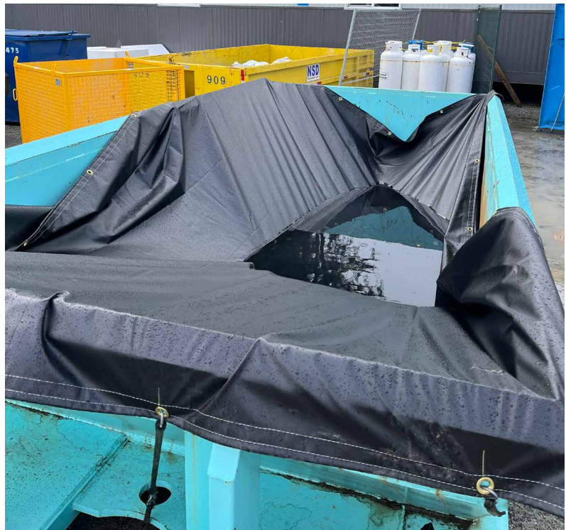
Figure 29: Water pooling on a lid of a plastics bin
