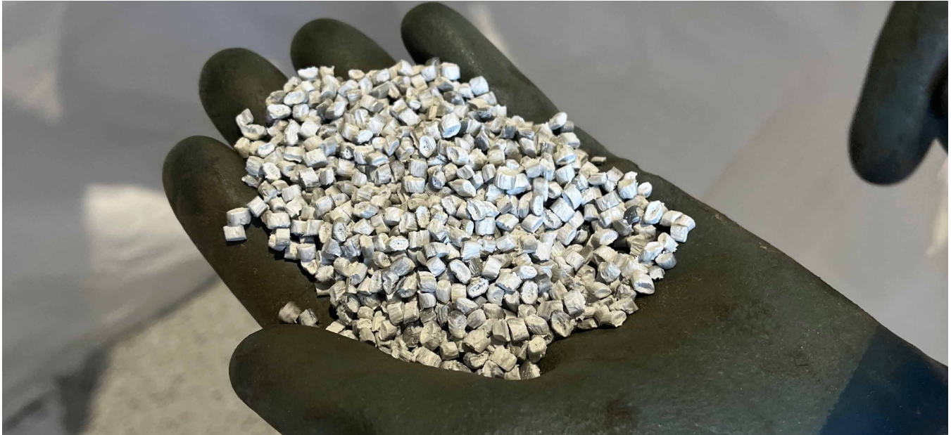
Figure 10: Pelletized plastic from construction sites
