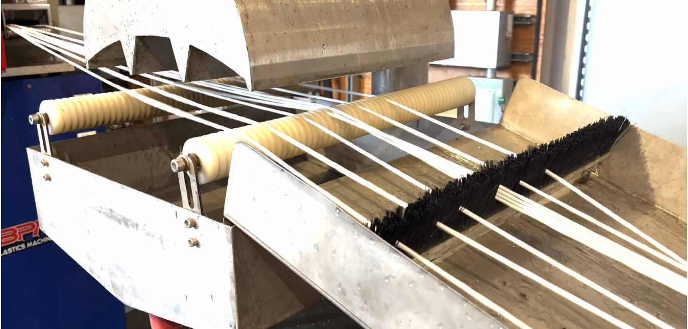
Figure 35: Construction plastic during extrusion
