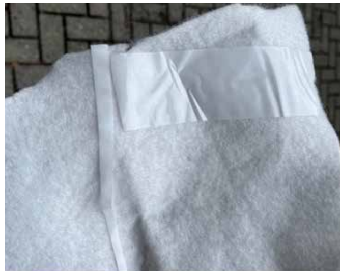
Figure 20: Non-woven polypropylene protective fabric (PP)
